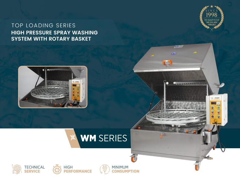
The parts which will be washed are placed on a basket that is placed on a stainless rotary platform with sliding system are washed in a closed cabinet with high pressured hot and detergent water. The washing process is done through water nozzles which are timed and compressive according to part structure, dirtiness rate; they clean the waste, oil, and chip on dirty surfaces in various angles.
